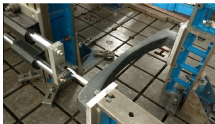
Fig. 21. The strength experiment of the bumper system.
