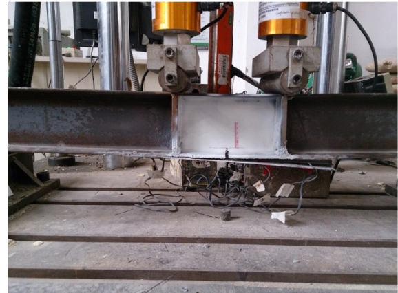
Fig. 19. Typical failure mode (specimenAR-3).
