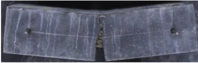
Fig. 4. Typical failure mode of UHPFRC beam (S19.5).
