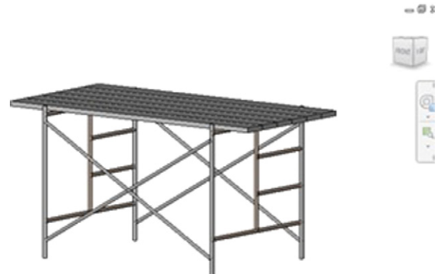
Fig. 4. Revit model of frame scaffold.
